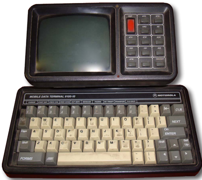
Figure 1-31 Mobile Data Terminals
